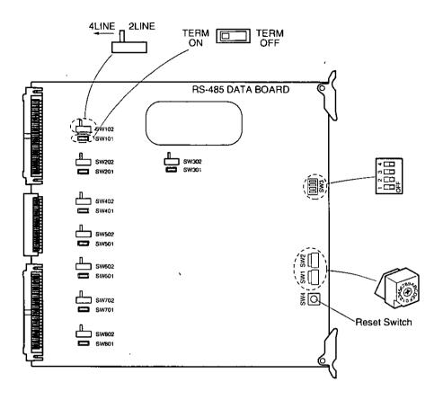
1. Set switches (SW1 and SW2) on the board to designate the RS-485 Data board number as shown in the following table. The factory default setting is Board Number 1 (00).
